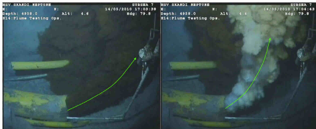
Figure 7 – Video capture of different colored fluids being discharged from the Riser End (arrow indicates trajectory)
