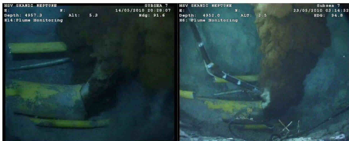
Figure 4 - comparison of second peak on 5/14 (Left) with stabilized stratified flow on 5/23 (right) 3 .
