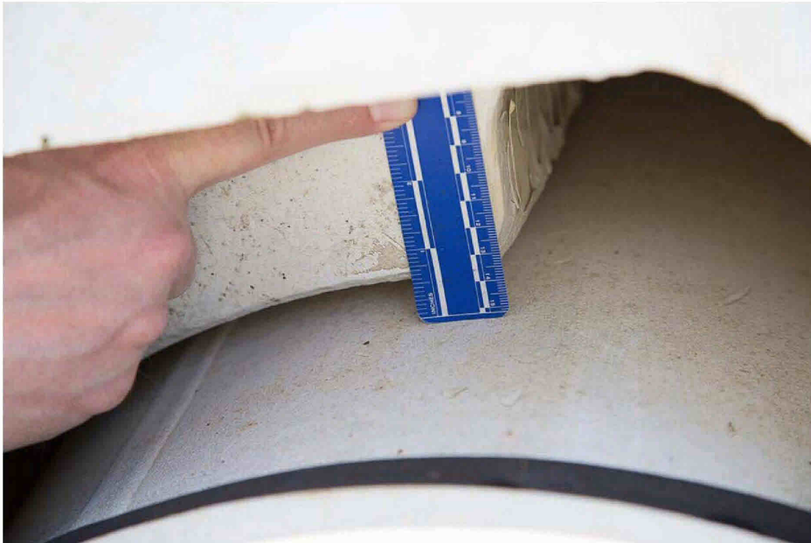
Figure 4 – Picture of riser strapped with buoyancy module showing gap between pipe wall and module 7
