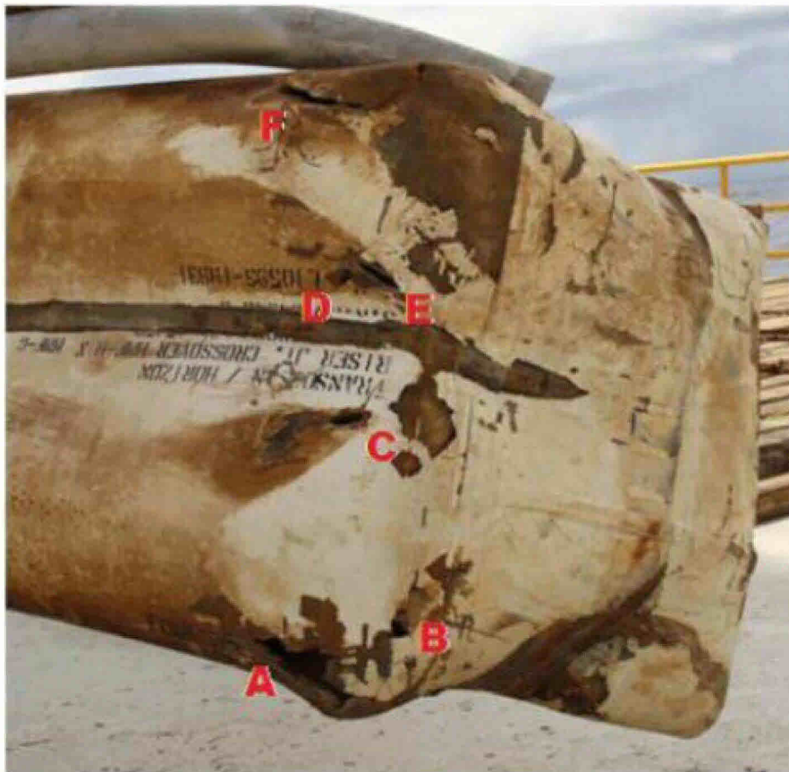
Figure 17 – Riser Kink annotated with labels for each hole in riser 23
