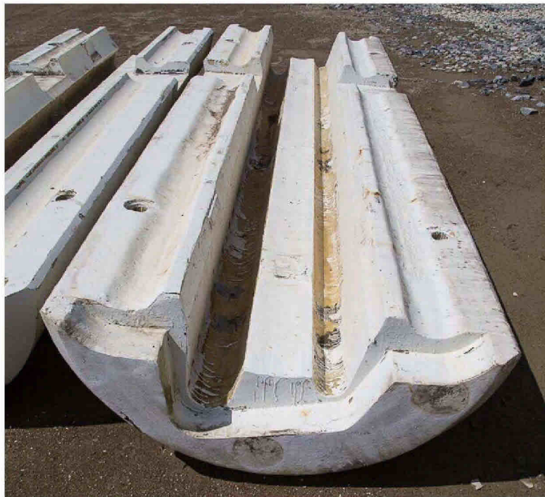
Figure 1 - two halves of DWH buoyancy modules 5
