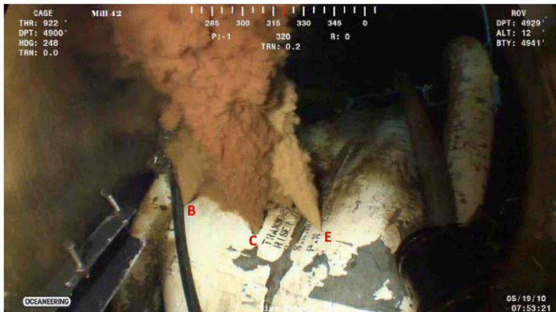
Figure 19 – Kink on May 19 showing only holes B, C and E leaking. 25
