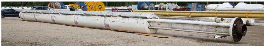
Figure 2 -Riser Joint with 5 of the 6 buoyancy modules 6
