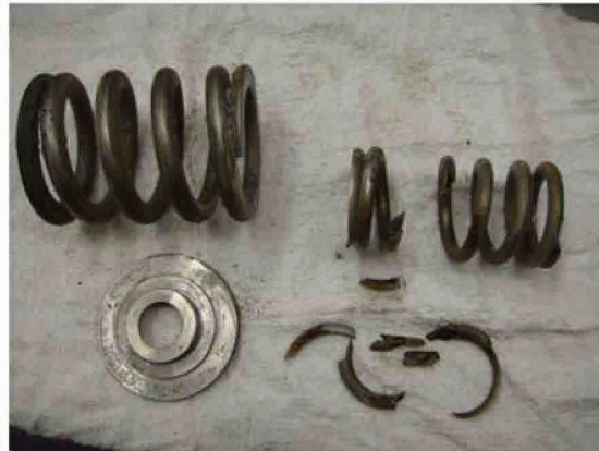
Figure 4.2: Shows the HP Casing Shear Close SPM dismantled.
