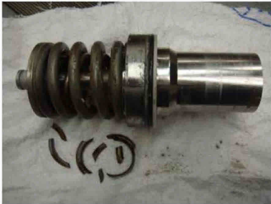
Figure 4.1. Shows the HP Casing Shear Close SPM with broken arbor spring.
