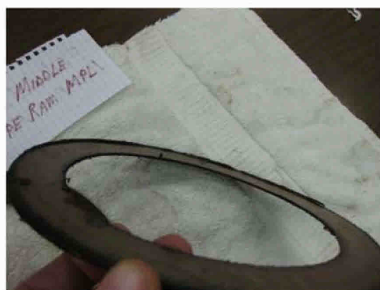
Figure 5.1: The aft middle pipe ram MPL locknut bearing that was replaced.
