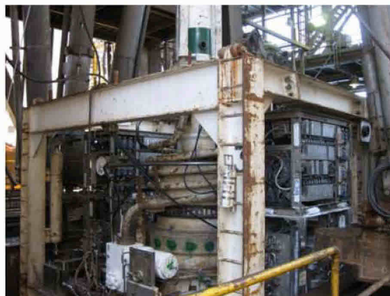
Figure 12.1: LMRP captured in the moonpool spider beams.
