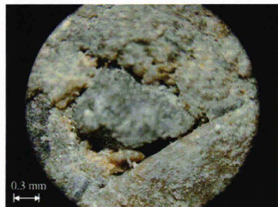
Fig. 11. The cracks on the interface of the aggregate and cement paste with w/cm=0.50.
