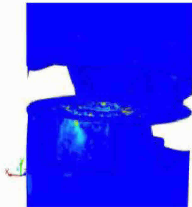
Figure 19. Erosion rate of eroded BSR assembly; red color indicates high values.
