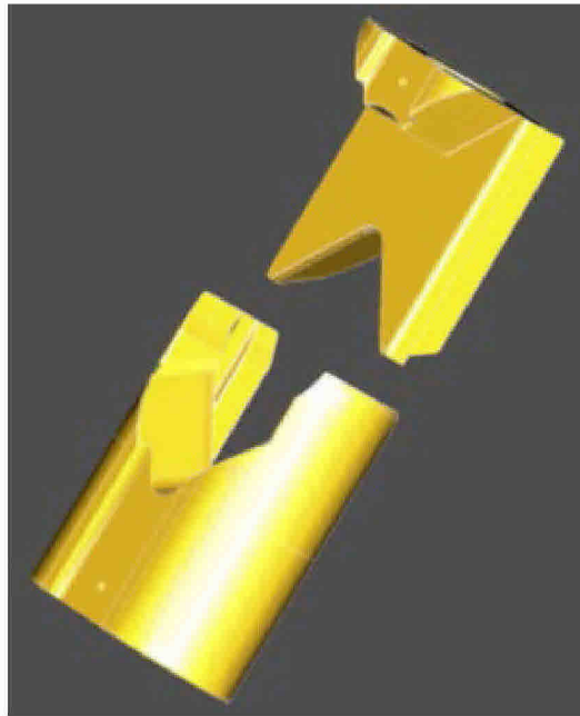
Figure 50. CAD model of pre-erosion CSR blocks.
