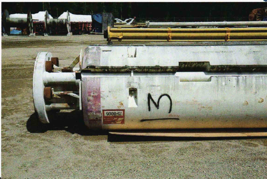
Figure 2 – A buoyancy module-covered riser joint similar to those used on Deepwater Horizon 3
