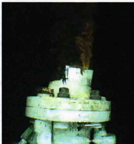
Figure A.3 Representative flow image from the top of the Macondo Well BOP after removal of the kinked riser section.
