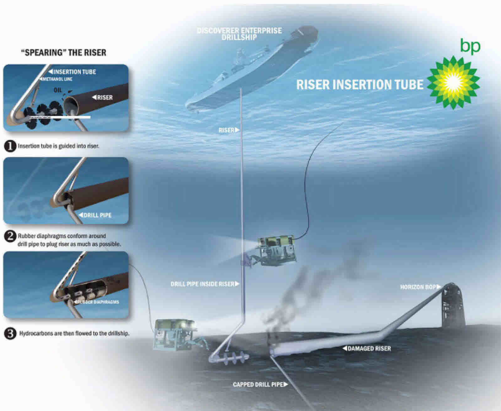
Figure 3. Diagram of Riser Insertion Tube Tool (RITT) that was used in mid-May to capture hydrocarbons being released from the open end of the damaged riser at the Macondo well spill site. Source: BP web.
