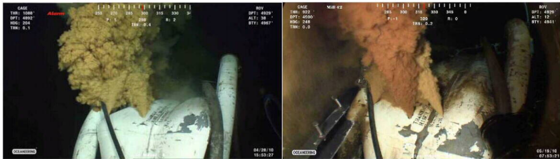
Figure 3 – Two holes on the Kink on April 28 (left) and three holes on the Kink on May 19 (right)
