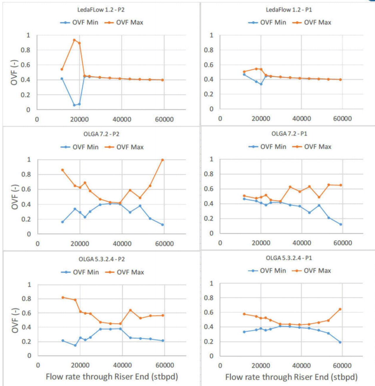
Figure 8 - OVF Bifurcation Map for hydrodynamic slug modeling using LedaFlow, OLGA 5.3.2.4, and OLGA 7.2
