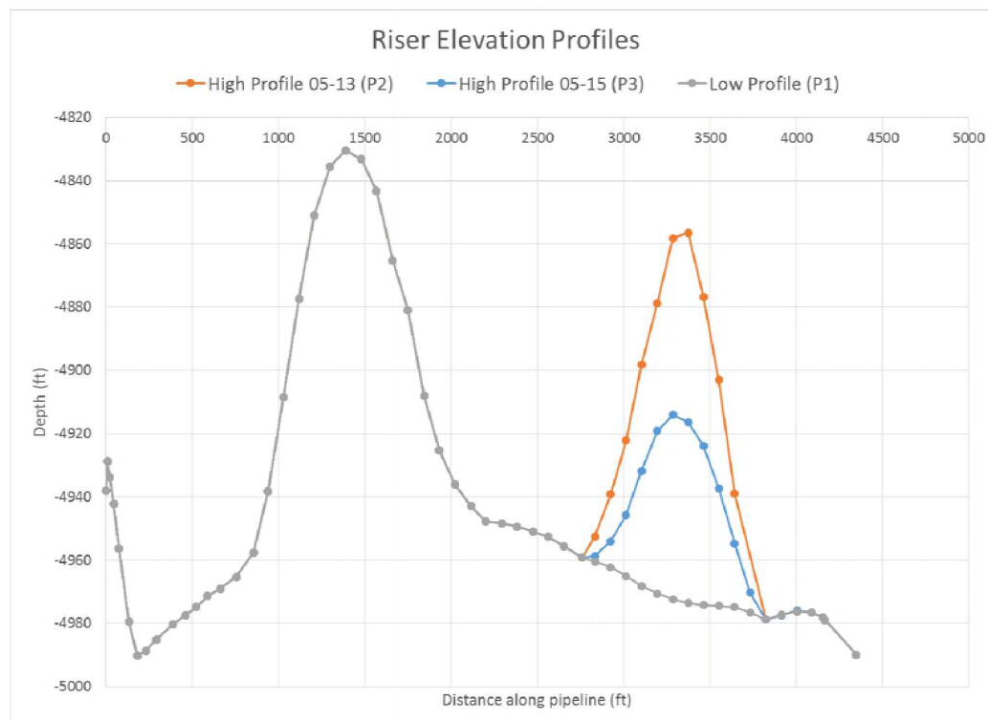
Figure 4 – Elevation profiles P1 (settled position), P2, and P3 (peak positions)
