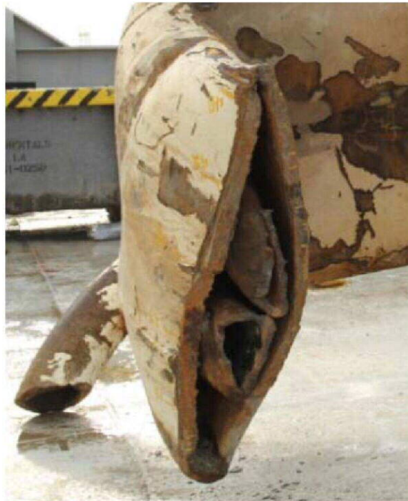
Figure 2 – Upstream section of the removed riser segment
