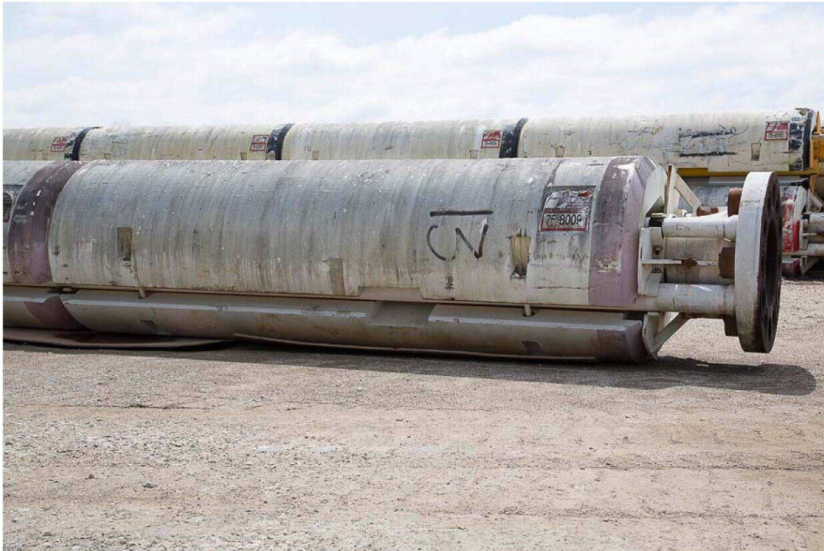
Figure 3 – Picture of buoyancy module-covered riser joint showing exposed pipe near the end 7
