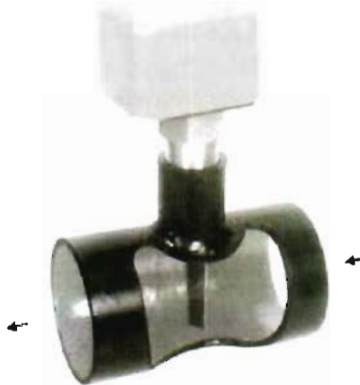
Figure 14: Typical paddle flow sensor, likely similar to Transocean's flow-out sensor
