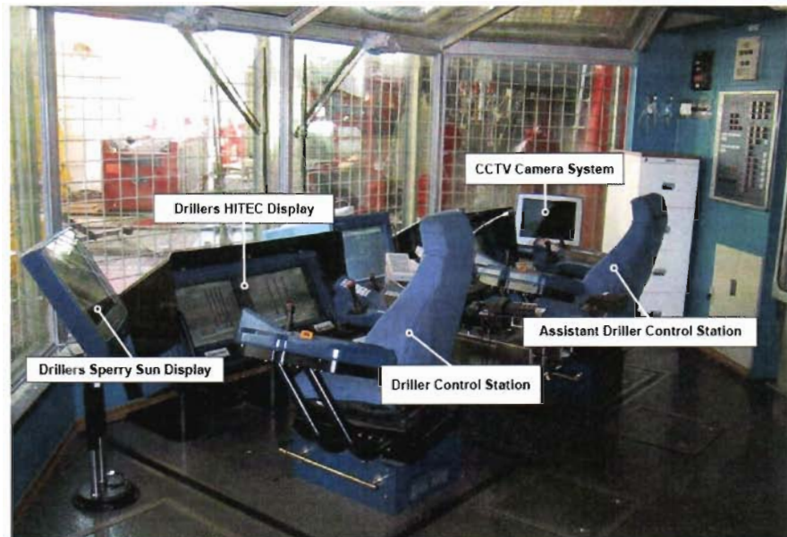
Figure 3: The Driller and Assistant Driller had access to both the InSite and Hitec Systems 14
