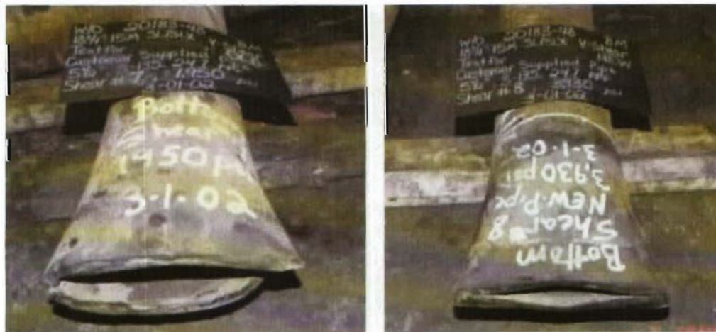
Fig. 9—Nearly 2,000 psi of increased pressure was required to shear the more ductile sample on the right. Both drillpipe samples were equivalent OD, wall thickness, and grade (West Engineering).
