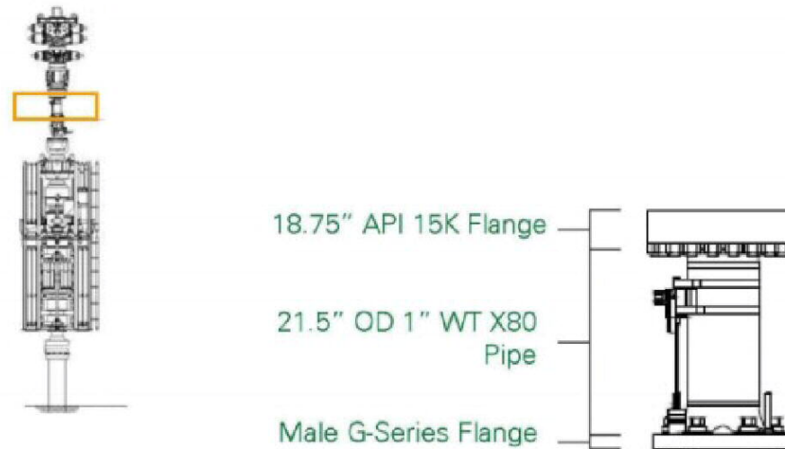
Figure 13 - Transition Spool Components
