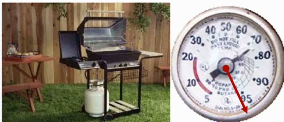
Figure 3.2. A schematic of material balance using a barbecue propane tank as an analogy. The gauge records the fraction of gas remaining in the tank. At the end of the incident, I calculate that the Macondo oil gauge read 97.1% (shown by the red arrow): 2.9% of the oil connected to the well had been released. This represents a pressure drop of almost 1,400 psi.
