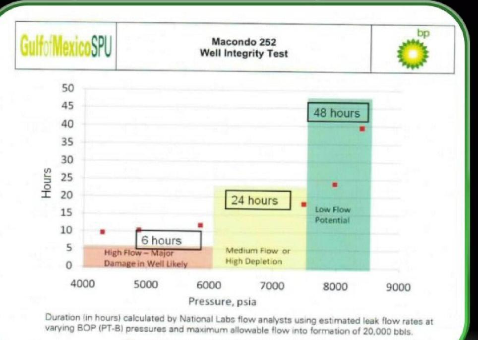
Figure 2: Well Integrity Test Duration Guidance
