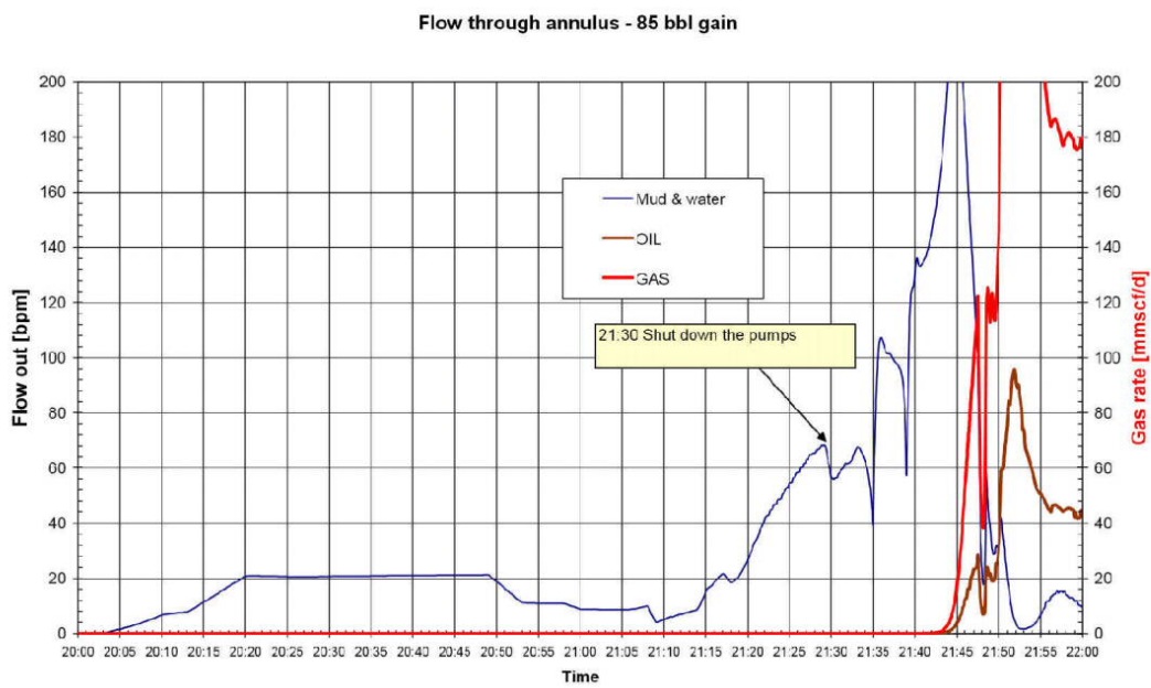
Figure 3.14: Case 2 - Flow through the outer annulus assuming 12.6 ppg sand and 86 ft reservoir exposure. Simulated flow rates at surface
