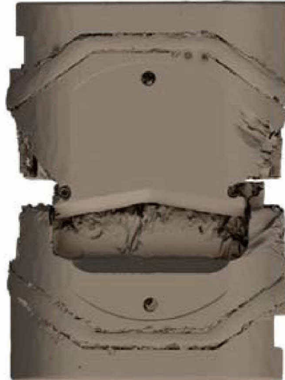
Figure 11 DWH SBR Ram Blocks, Top View
