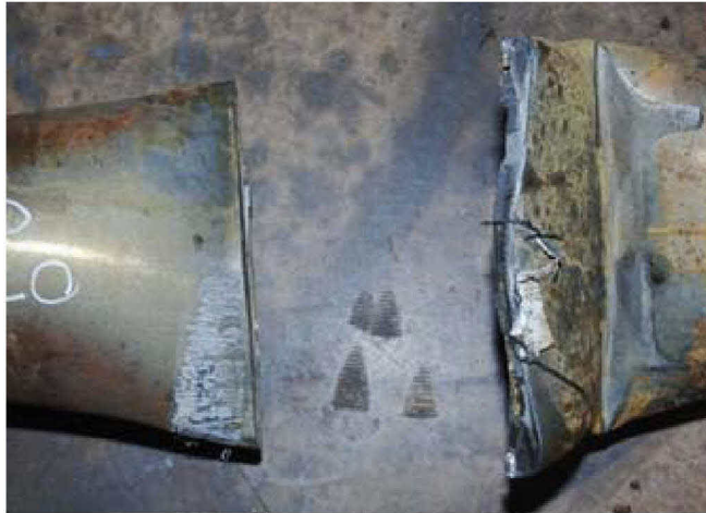
Figure 7 Normal Shear: Ends Display Uniformity, Symmetry
