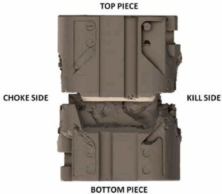
Figure 9 Closed DWH SBR Ram Blocks, Bottom View
