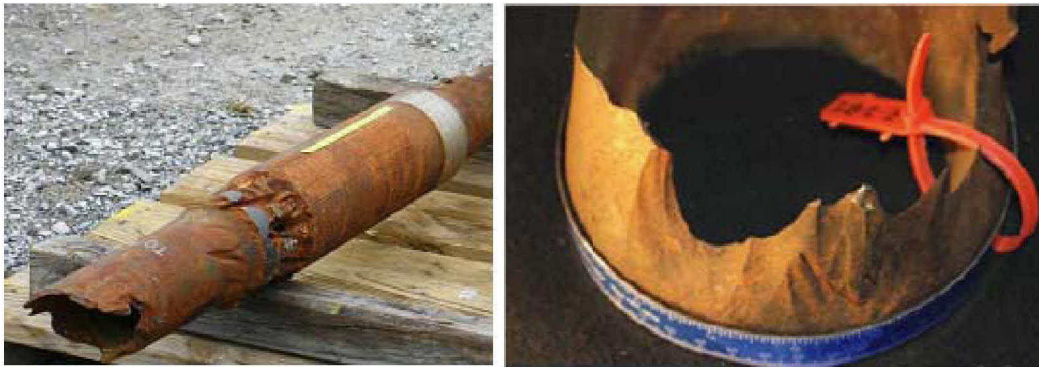
Figure 5 Picture of “Tool Joint A” and Upper End of Segment 1-B-1.
