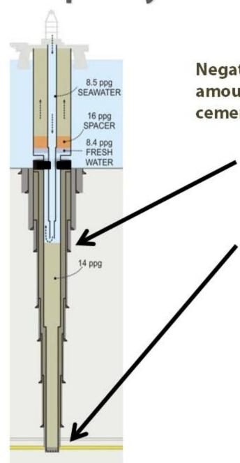
Negative pressure differential must equate to full amount of planned underbalance to be "seen" by the cement shoe at the base of the well.
