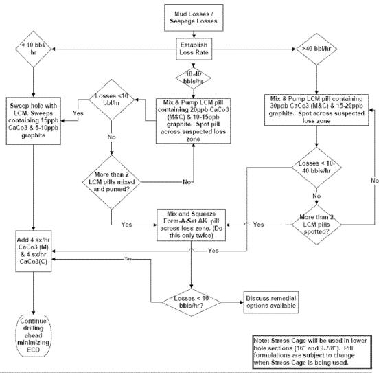
Note: Avoid Rapid movement of pipe causing surge pressures while circulating. Avoid rapid pump start up. In suspected loss circulation intervals, have 300-400 bbls of loss circulation pill ready consisting of: 10 lbs/bbl G-seal, 20 lbs/bbl Safe Carb 40, 20 lbs/bbl Safe Carb 250, 20 lbs/bbl Vinseal
