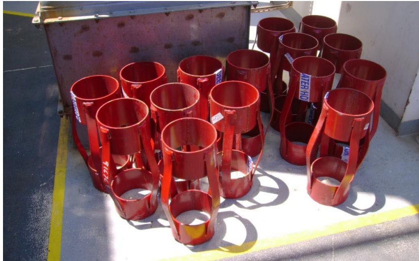
Figure 4-3. Photograph of centralizers delivered to the Deepwater Horizon .
